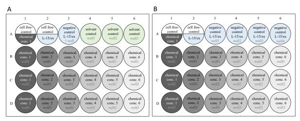
Figure 5: Pipetting scheme for a test chemical (one test chemical, six test concentrations and three technical replicates per concentration with "conc. 1" signifying the highest test concentration). Panel A represents a pipetting scheme for a test chemical where an organic solvent is used for exposure solution
