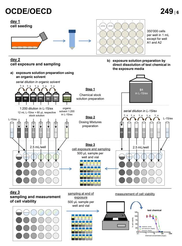
**Figure 2: General overview of the test procedure.** S1 to S6 refer to the test chemical stock solutions that are used for the preparation of dosing mixtures in the final test concentrations C1 to C6, with S1 and C1 being the highest concentration, respectively. For detailed information on the pipetting scheme of a test chemical, see Figure 5.
