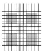
Figure Annex 4-1: Simplified picture of the counting areas of a Neubauer chamber. Areas for counting are marked grey. The number of cells in each grey quadrate is noted.
