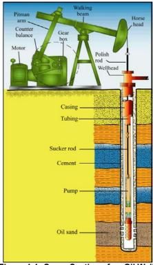
Figure 1-1: Cross-Section of an Oil Well
