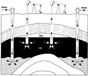
Figure 2-1: Example of Secondary Recovery
