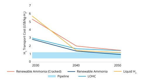
**Source:** Authors' elaboration and projection based on data from Saygin (2023), IRENA (2023), and IEA (2023). **Note:** The pipeline transport cost assumes a 2,000 km pipeline with the lower range representing the costs of retrofits and the higher reflecting the end of the pipeline cost showing the costs of installing a new pipeline.
